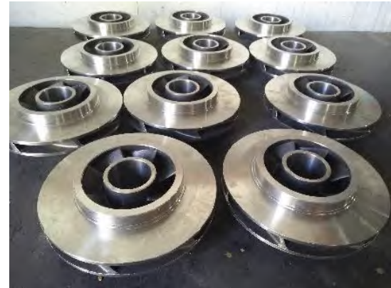
Duplex investment casting-230 mm Q = 100 m 3 /hr P=40 bar (5 stages)
